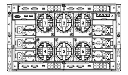
Base BladeSystem c3000 Enclosures ship with four fans installed, supporting up to four half-height devices or two full-height server blades. Adding two additional fans to the enclosure allows population with eight half-height devices or four full-height server blades.
